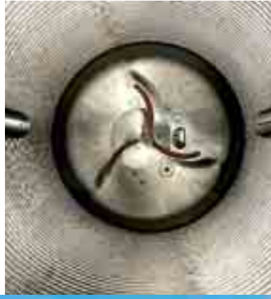
Inside view of a PVC high-performance reactor
