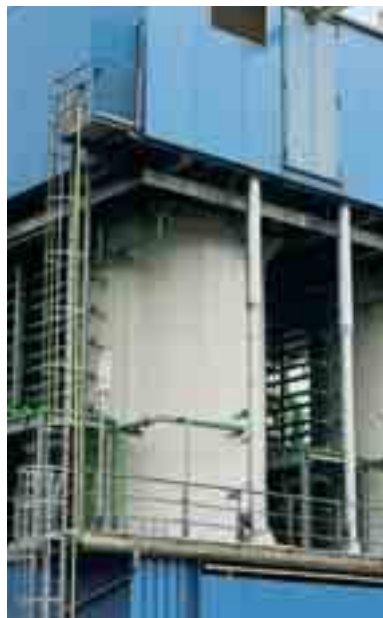
PVC high-performance reactor 115 m 3 volume
