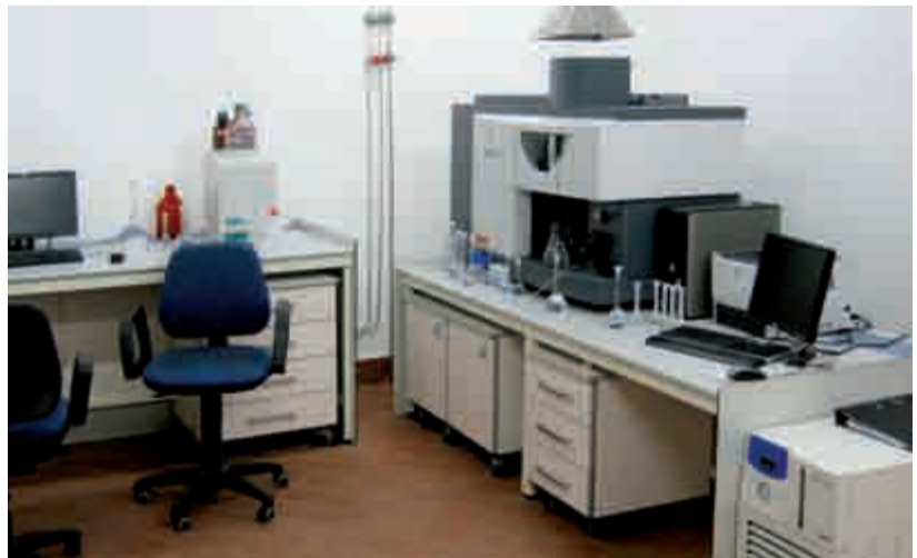
Laboratory after installation: ICP
